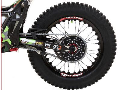
Factory Spec Machined Rear Wheel Rim: In anodised black finish.
