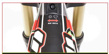
**New Location Of Mapping Switch:** Which is now incorporated into the airbox cover. This allows the rider to switch between maps with ease.
